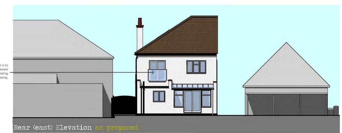
New glass balustrade set in to Anodised aluminium channels fixed either side of existing opening.
